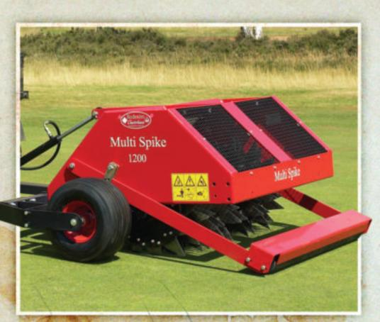
For general aeration, the standard 1/8" (3mm) thick triangular knife will give you 8" (200mm) deep slits at a close 6" (150mm) spacing, while the fine slitting drum will give you 4" (100mm) deep slits at an extra close 3" (75mm) spacing.
