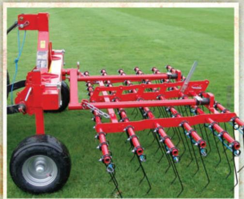
The Verti-Rake decompacts turf surfaces using thin spring-loaded flexible tines.
