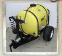
The Redexim Trailed Sprayer is an excellent tool for any turf spray application. Easily coupled to most any tow vehicle, the 12 volt sprayer quickly disperses up to 65 gallons of Redexim ATD (artificial turf disinfectant) and other liquids such as static reducing mixes, or plain water to cool the playing surface.
