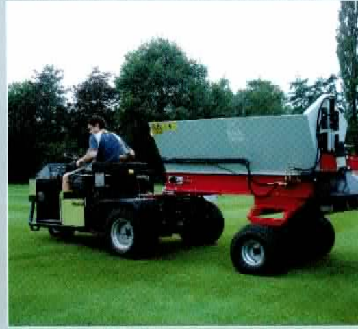
The Rink DS 800 can be carried either on top of the utility vehicle (above) or be pulled (below)
