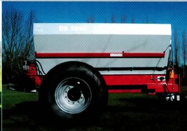
The DS 3800 spreads the material up to 15m (6½ ft) wide
