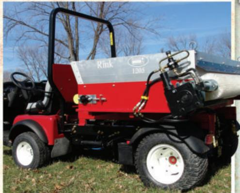
The 12 series top dressers offer you the widest brush applicator top dresser available with a smooth even spread, over 6 ft. wide. This makes the 1205 body mount spreader ideal for fitting onto your utility vehicle, as its spreading width will be outside the vehicle's wheel width.
