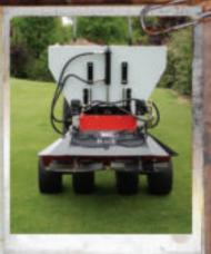
The Rink DS 1200 is a topdresser with dual spinners with a spread pattern variable up to 30 ft (10 m). The operation of the belt and spinners can be done from the tractor seat, by switching the hydraulic lever. No unnecessary drop of material takes place between stopping and operation, since the material release gate automatically closes when the belt is stopped. The spinner disks have been designed in a way that they will handle wet material very well.
