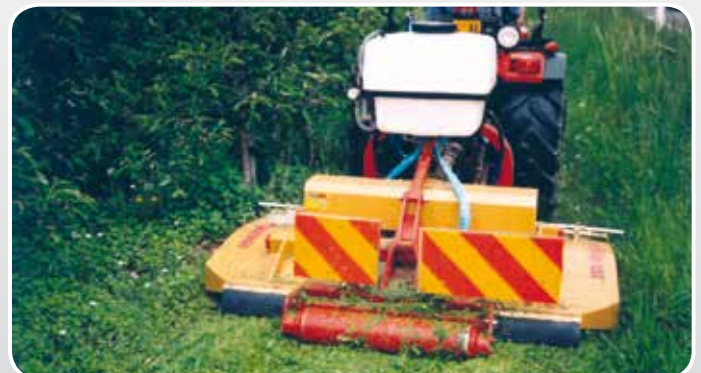
The herbicide spraying system XID may be mounted to many SEPPI mowers. High-precision nozzles come with adjustable spraying direction.
