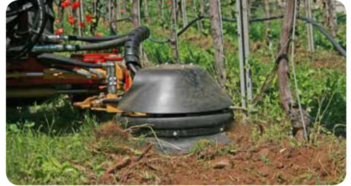
The cultivator XSA supports organic agriculture. A mechanical process cuts the roots of weeds and brings them to the surface.
