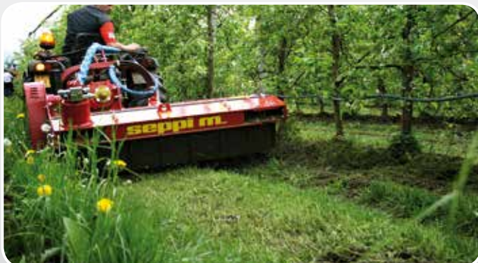
The conveyor belt XTR deposits grass to the right of the mulcher. This inhibits the growth of the grass and allows to reduce the use of chemicals.
