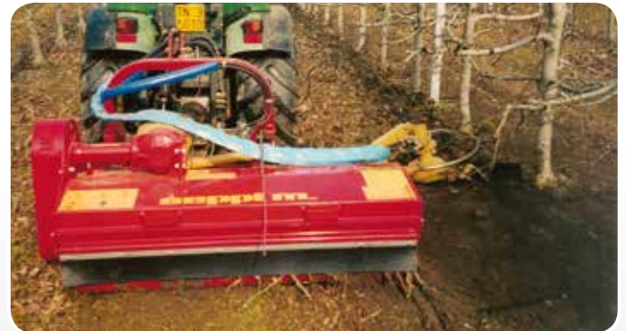
With the sweeper XAN you may collect leaves and prunings from row sides and bring them into an ideal position for mulching: in front of the mulching mower.
