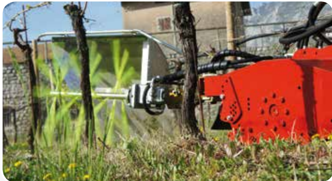
The brushes of the shoot remover XSP clean the trunk and remove shoot, suckers and straw mechanically – without chemicals.
