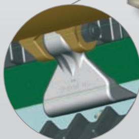
SMO flail with double counterknives inside the frame
