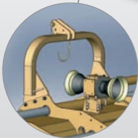
easily changeable hitch to change the working direction
