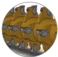
fixed knife rotor with tungsten tips
